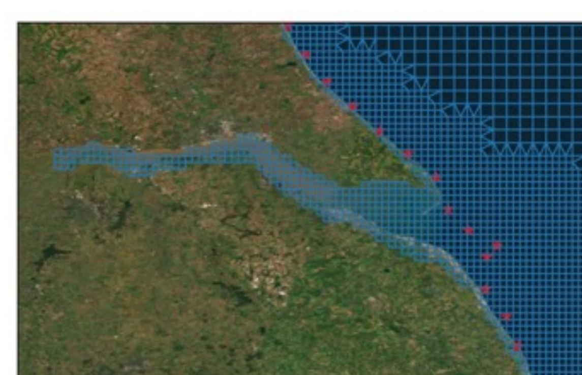
Figure 7: The tide and surge model Delft3D-FM with increasing resolution in the Estuary
