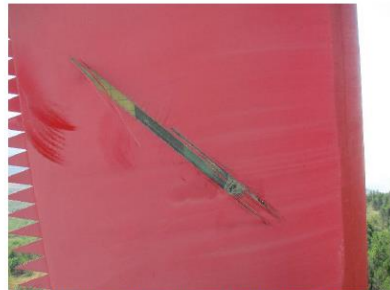
Photo 1: Damaged laminate by lightning strike. SS. Z47,2m
